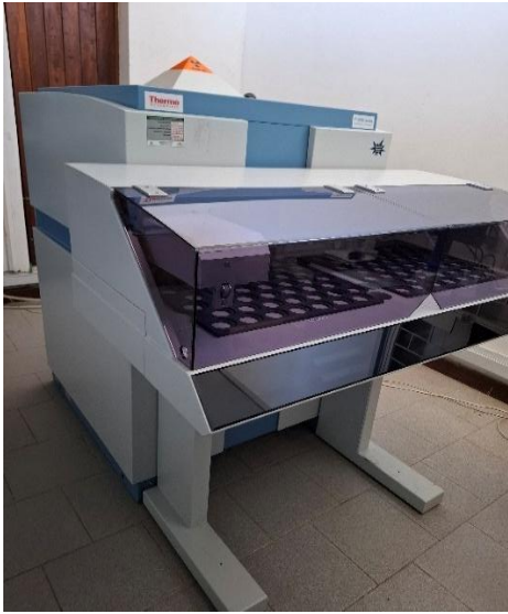
Photo 5.1: Bench XRF - Photo taken by the audit team during a site visit at the Mining Commission's Mineral Laboratory on 7 October 2025.
