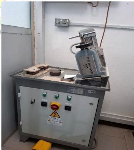
Photo 5.4: Cupel Sample Treatment Unit - Photo taken by the audit team during a site visit at the Mining Commission's Mineral Laboratory on 7 October 2025.
