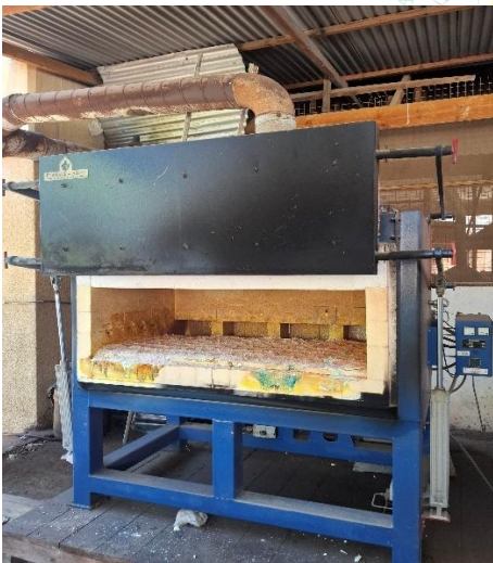
Photo 5.3: Fusion Furnace & Assay Supplies - Photo taken by the audit team during a site visit at the Mining Commission's Mineral Laboratory on 7 October 2025.
